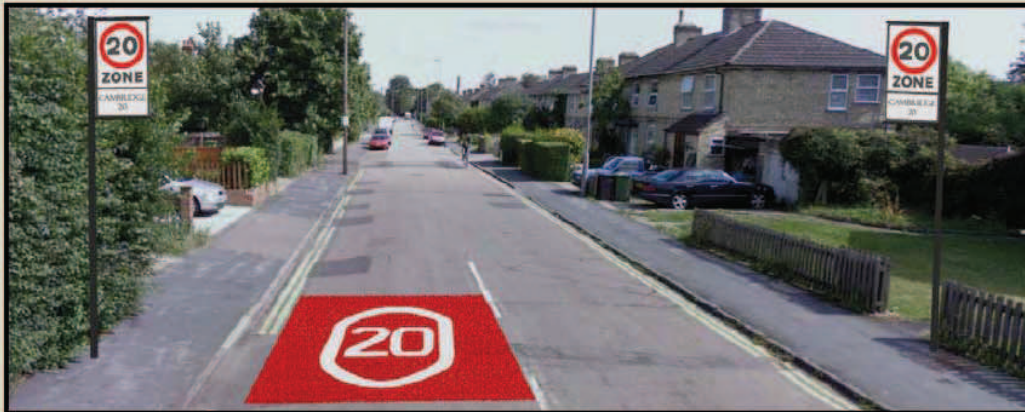
Example of how entry into the proposed 20mph on a main road could look: a 20mph 'roundel' road marking with coloured road surface and two 20mph Zone entry signs.
